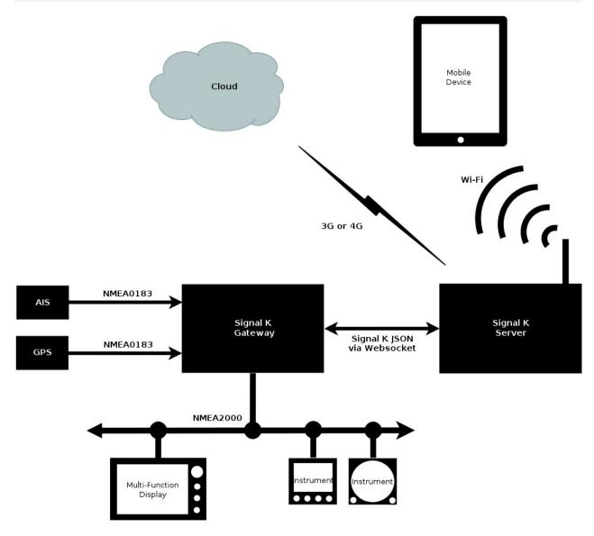
One major advantage of Signal K is the ability to represent data from heterogeneous sources. In addition to traditional NMEA sources, data from generic sensors as well as modern Signal K enabled sensors can be fused into a single data model and a single protocol for accessing the data. Another typical configuration is a Signal K server with adapters and converters for the different sources.
